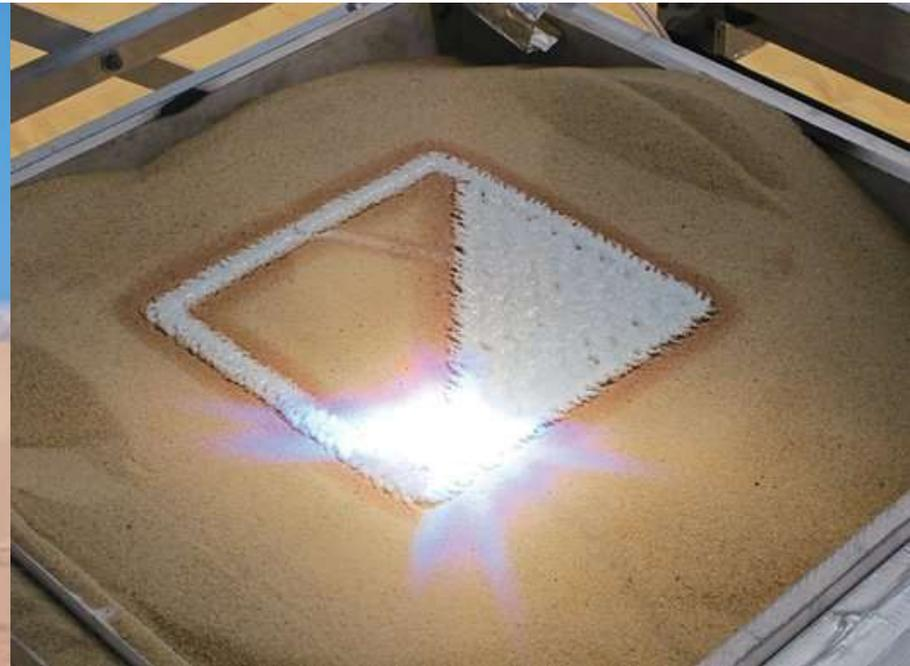
Markus Kayser's "Solar Sinter" 3D printer
