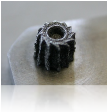
A 12-edge micro-reamer in SS AISI420 for a biomedical device.
